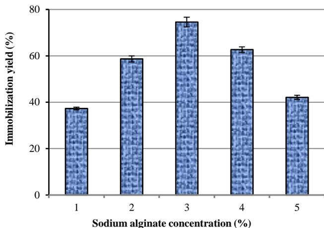
Figure 1 Effect of Sodium-alginate concentration on immobilization efficiency
