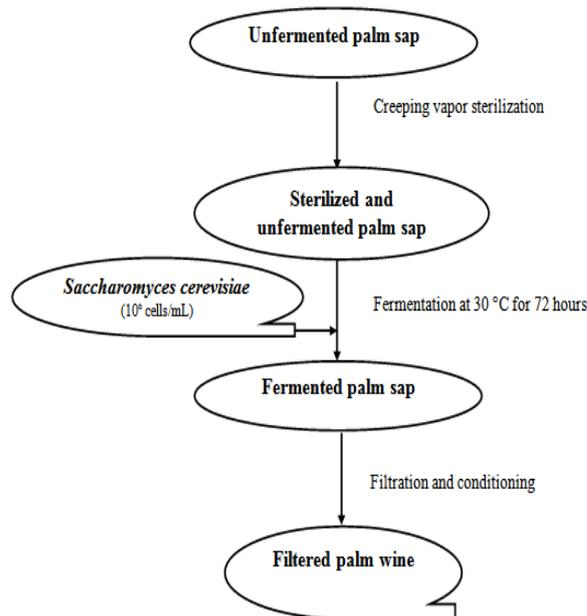
**Figure 3** Flow chart (diagram) for controlled fermentation of palm wine
