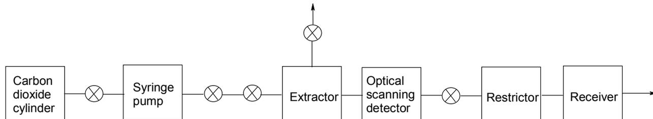
**Figure 1** Schematic drawing of SFE apparatus
