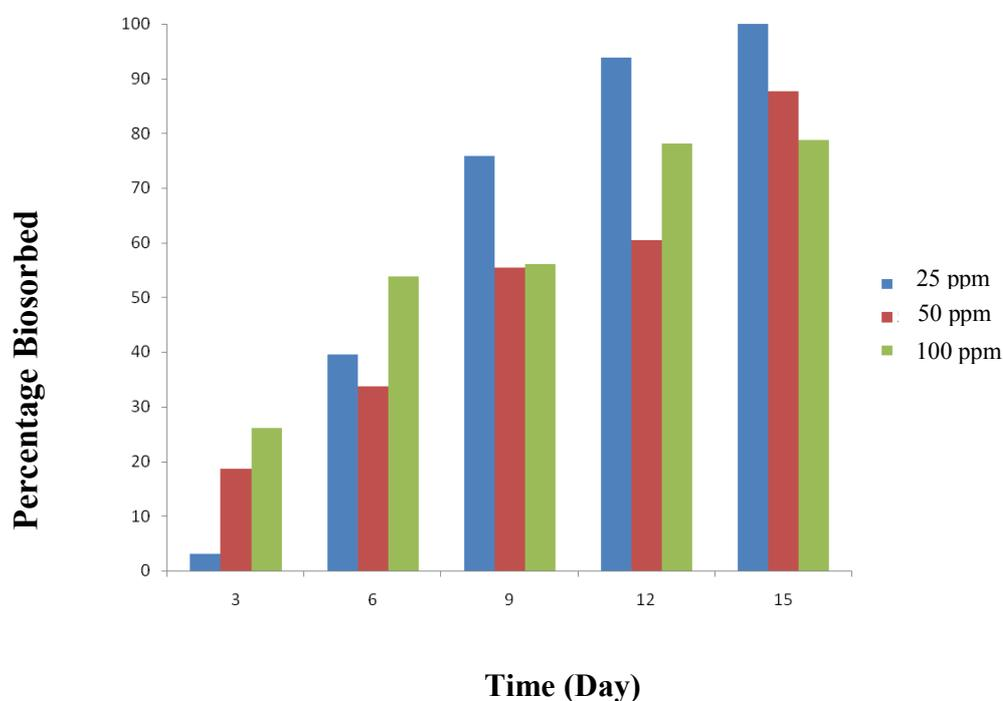
**Figure 2** The variation in bioaccumulation capacity of *T. longibrachiatum* with time at various concentration of lead ion (at 25 °C and pH 4.)
