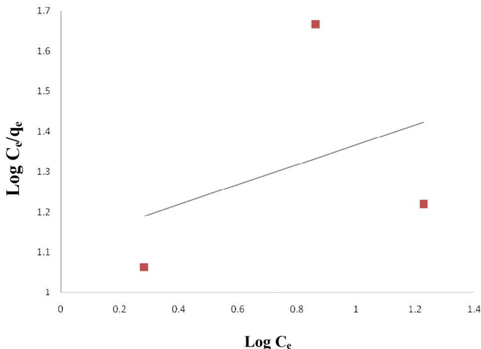
**Figure 5** Freundlich adsorption isotherm for the biosorption of lead ion on plumb shell at 25<sup>0</sup>C
