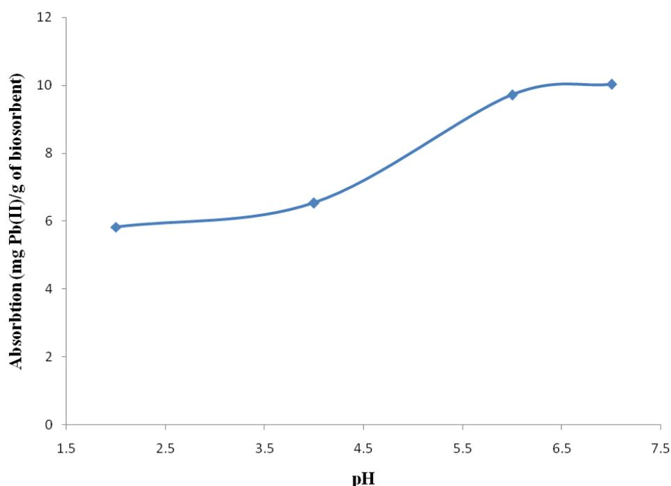
**Figure 6** Effect of pH on the biosorption of lead ion by *T. longibrachiatum*
