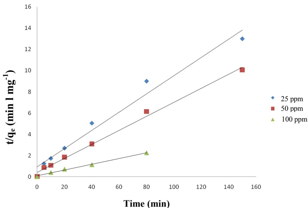
**Figure 3** Pseudo-second order kinetics for the biosorption of lead ion by *T. longibrachiatum* at 25 °C
