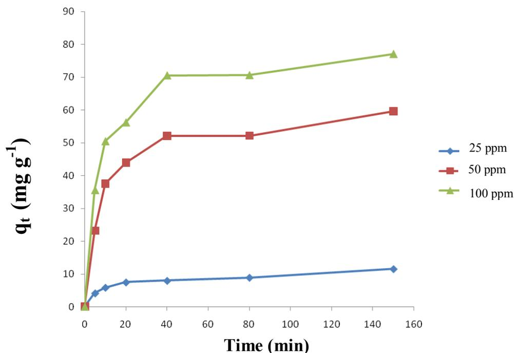
**Figure 1** The variation of adsorption capacity with biosorption time at various concentration of lead ion (at 25 °C and pH 4,)
