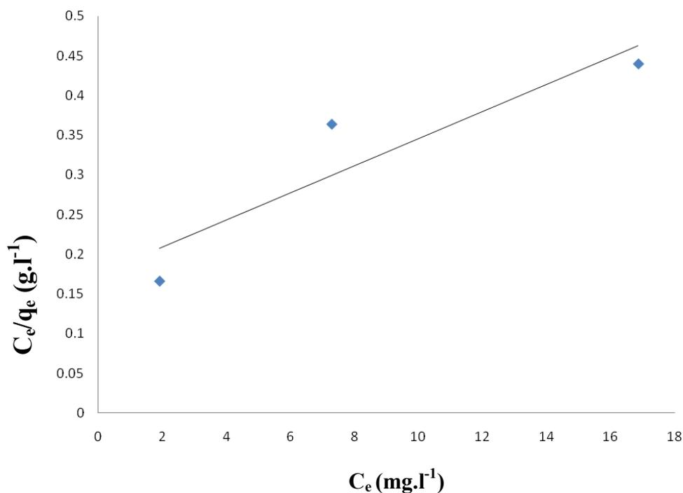
**Figure 4** Langmuir adsorption isotherm for the biosorption of lead ion on *T. longibrachiatum* at 25 °C
