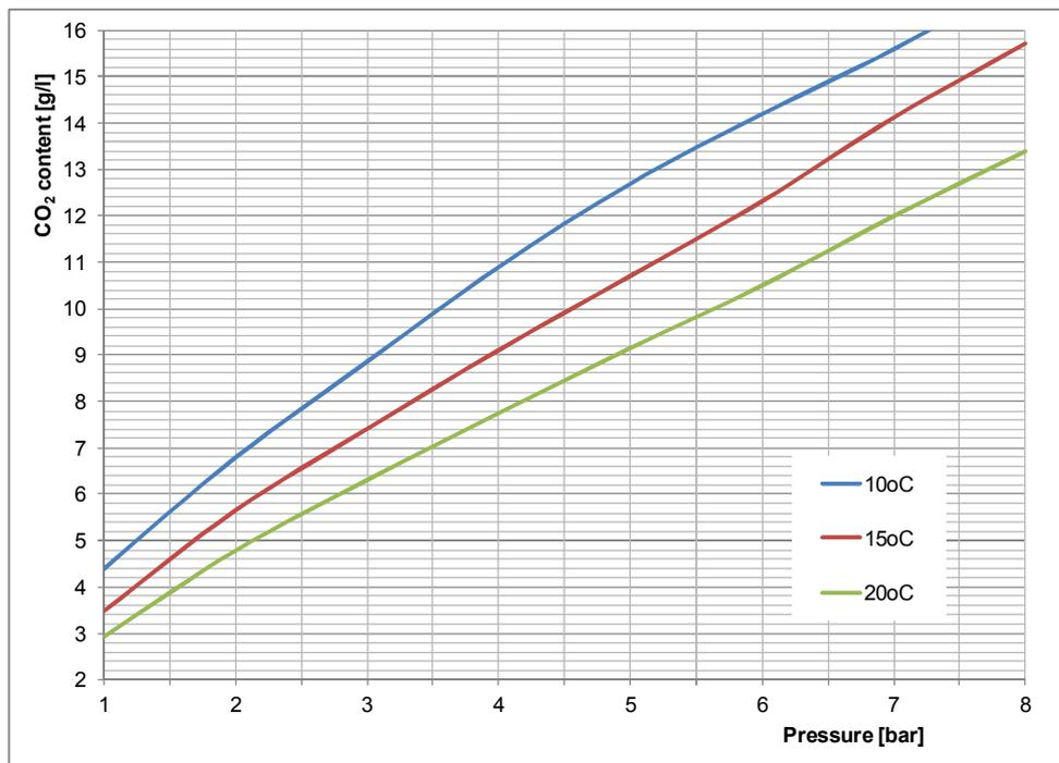
**Figure 3** Absorption of CO<sub>2</sub> as a function of the temperature and pressure
