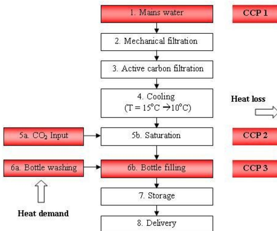
**Figure 2** The soda production process
