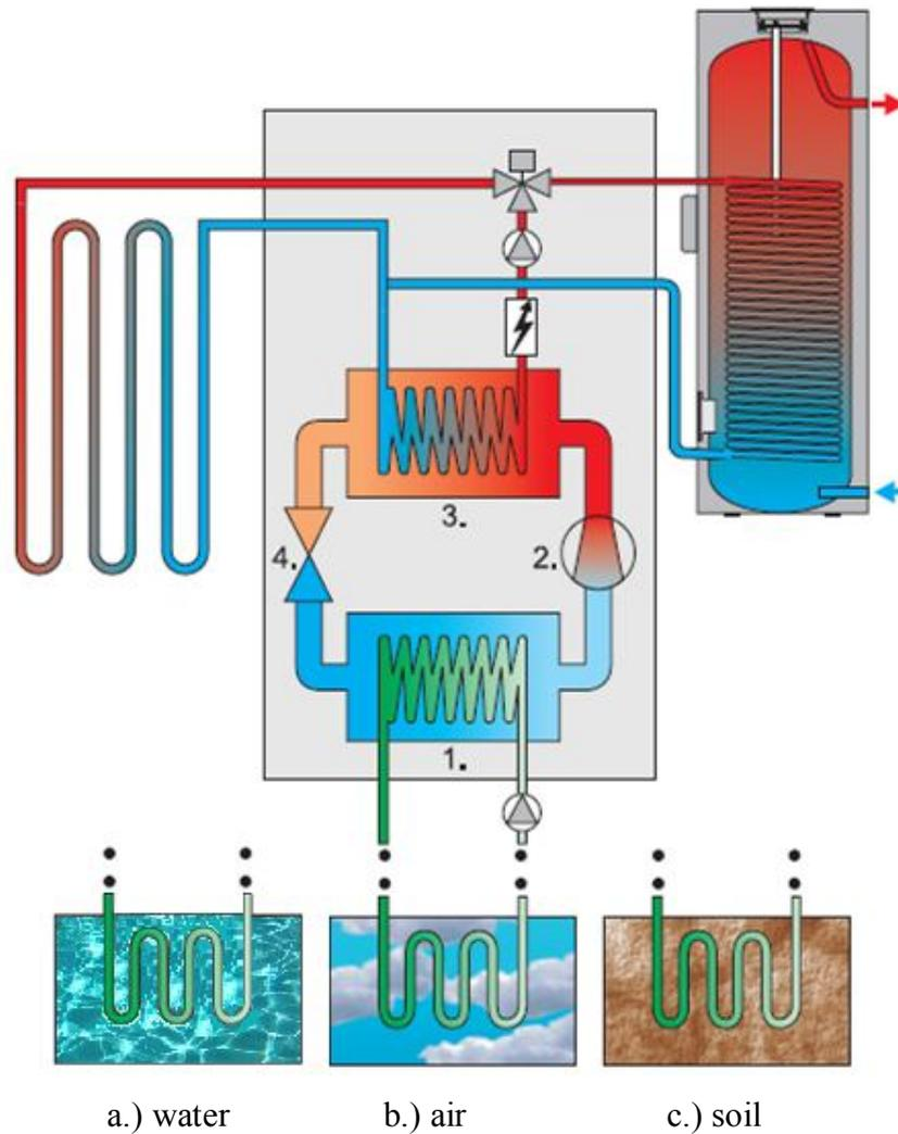
**Figure 1** Operation principle of heat pump
