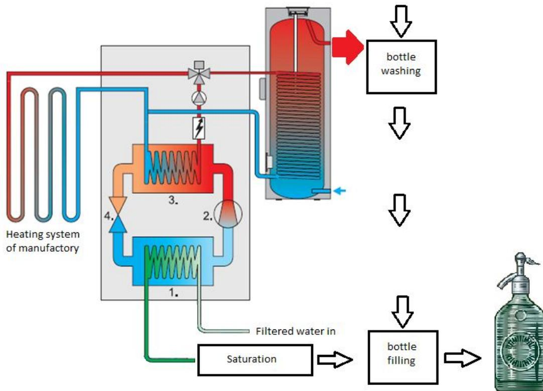
Figure 4 Heat pump in the soda process
