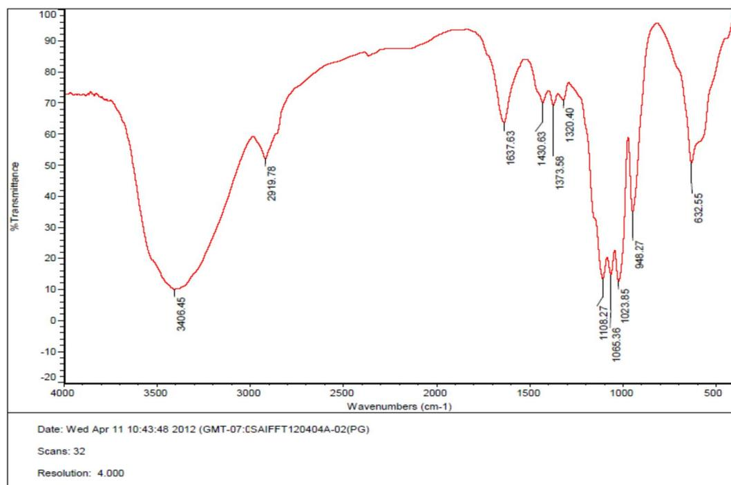
**Figure 3** FTIR analysis of extracted PHA from SPY-1
