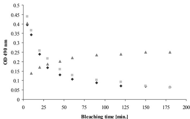
**Figure 2** The relation of the optical density at 490 nm (OD 490 nm) of the bleached oil on the bleaching time at various temperatures (♦ - 20, ■ - 50 and ▲ - 80 °C).
