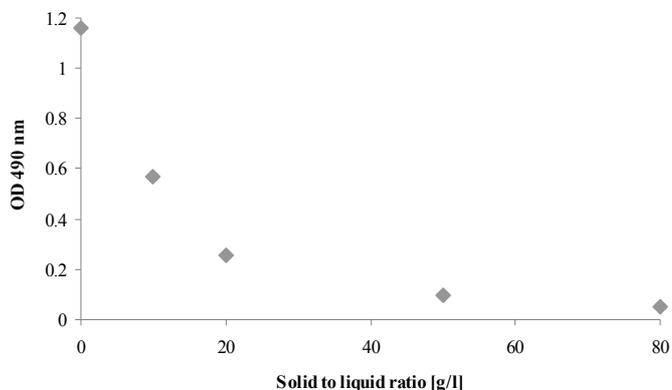
**Figure 1** The relation of the optical density at 490 nm (OD 490 nm) of the bleached oil on the amount of the added activated bleaching earth expressed as solid-liquid ratio parameter.
