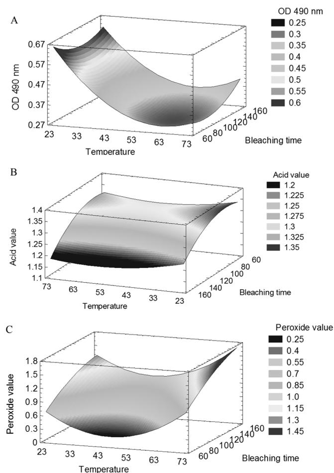
**Figure 3** The relation of the dependent variables (optical density at 490 nm, acid value and peroxide value) on the temperature and bleaching time at constant solid to liquid ratio, which were 33 g/L oil; A – optical density at 490 nm (OD 490 nm); B – acid value, expressed as mg KOH/g oil; C – peroxide value expressed in mmol O/kg oil
