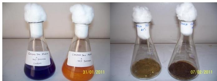
**Figure 1** Screening invertase activity using Fehling’s reagent **Figure 2** SSF using papaya peel substrate
