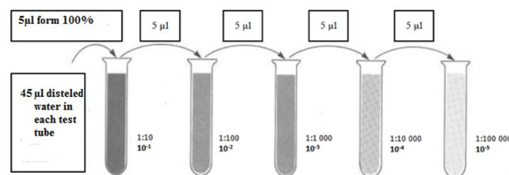
Figure 1 The standard procedure of decimal dilution with water
