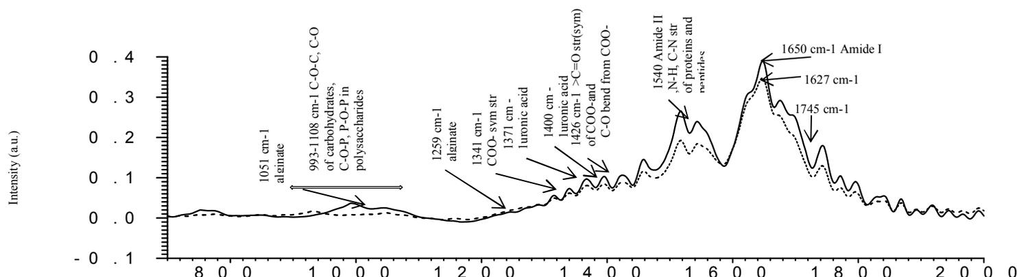
**Figure 1** Normalized FTIR spectra of planktonic (dotted line) and biofilm (continuous line) cells of *C.sakazakii*.
