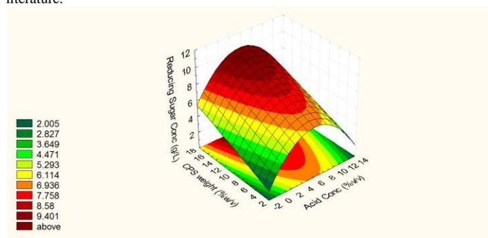
**Figure 6** Response surface plot showing effect of acid concentration and weight of CPS on the reducing sugar concentration released by acid hydrolysis of CPS
