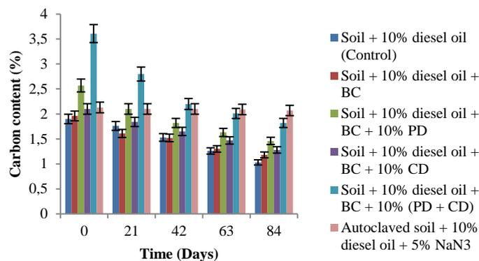
**Figure 4** Carbon contents of diesel contaminated soil during bioremediation
