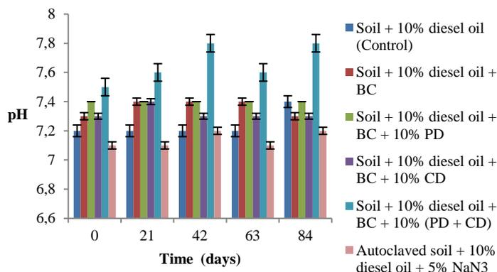
**Figure 1** pH values of diesel contaminated soil during bioremediation
