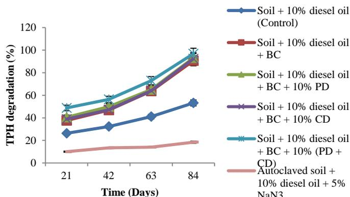
**Figure 7** Total petroleum hydrocarbon degradation in diesel contaminated soil during bioremediation
