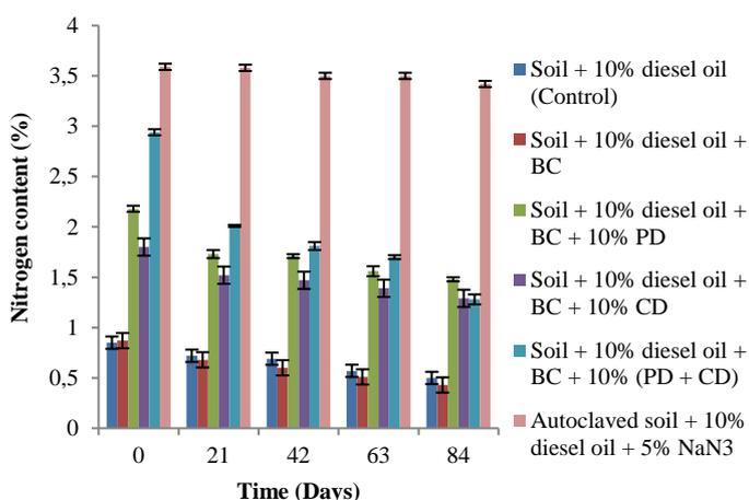
**Figure 2** Nitrogen contents of diesel contaminated soil during bioremediation
