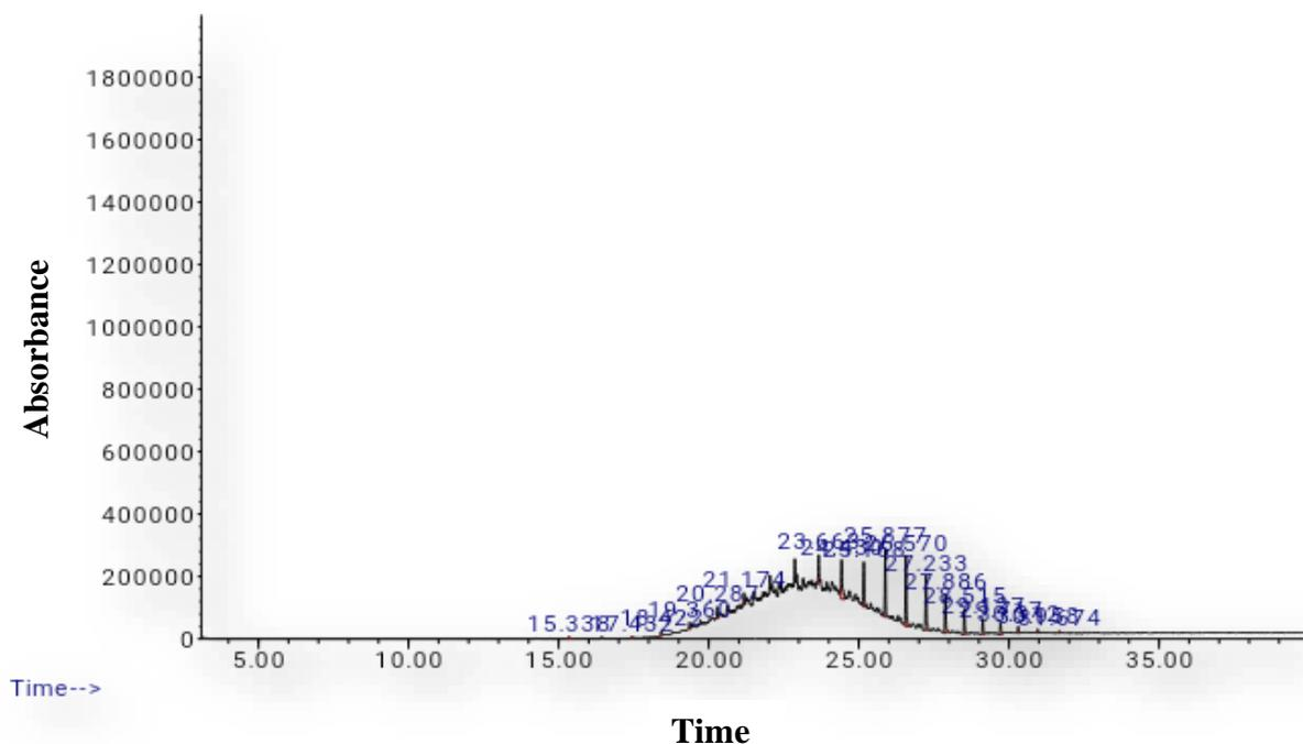
Figure 11 Chromatogram of diesel contaminated soil remediated with bacterial cocktail + 10% cow dung after of 84 days
