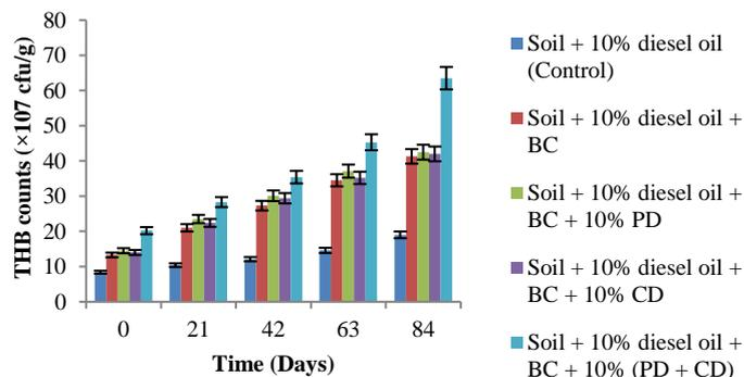
**Figure 5** Total heterotrophic bacteria (THB) count in diesel contaminated soil during bioremediation
