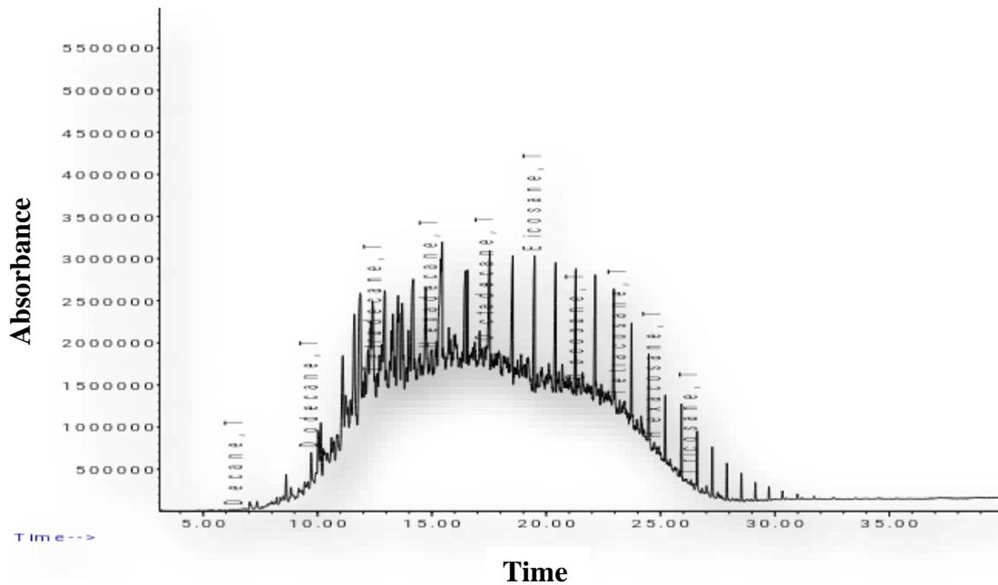
Figure 9 Chromatogram of diesel contaminated soil remediated with bacterial cocktail + 10% cow dung + poultry dropping after of 84 days
