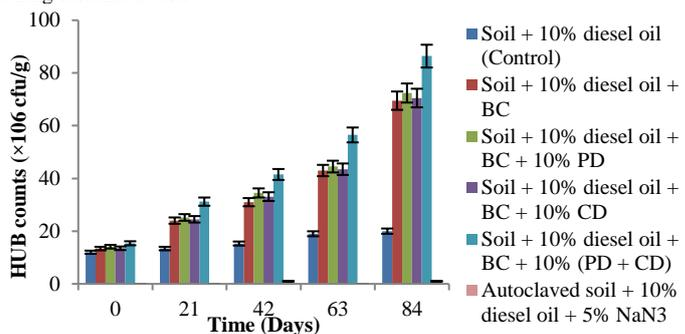
**Figure 6** Hydrocarbon-utilizing bacterial (HUB) counts in diesel contaminated soil during bioremediation
