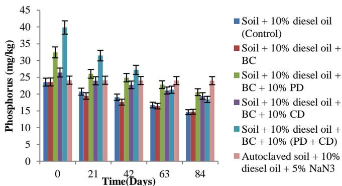
**Figure 3** Phosphorus contents of diesel contaminated soil during bioremediation
